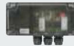
2-channel relay receiver HET-E2 24 BS NEW from July 2014 With 2 volt-free relay outputs for choosing the direction, a 2-pin input for volt-free Open and Close limit switch reporting, for querying the door position
